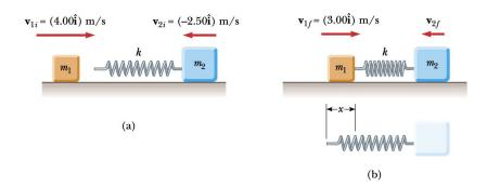
a) Find the velocities of the two blocks after the collision.
