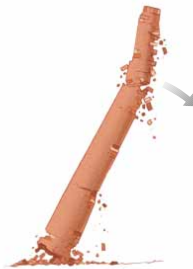
Figure 10.19 (Conceptual Example 10.11) A falling smokestack breaks at some point along its length.
