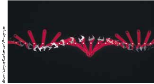
Figure 9.24 Multiflash photograph showing an overhead view of a wrench moving on a horizontal surface. The white dots are located at the center of mass of the wrench and show that the center of mass moves in a straight line as the wrench rotates.
