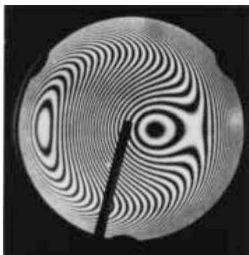
Figure 37.19 This asymmetrical interference pattern indicates imperfections in the lens of a Newton's-rings apparatus.
