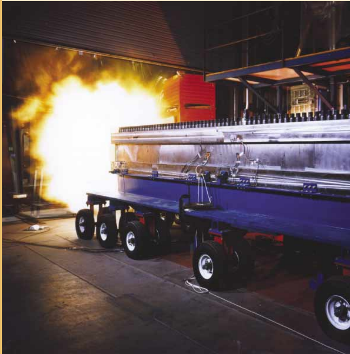
▲ A proposed method for launching future payloads into space is the use of rail guns, in which projectiles are accelerated by means of magnetic forces. This photo shows the firing of a projectile at a speed of over 3 km/s from an experimental rail gun at Sandia National Research Laboratories, Albuquerque, New Mexico. (Defense Threat Reduction Agency [DTRA])
