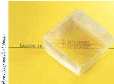
Figure 38.35 A calcite crystal produces a double image because it is a birefringent (double-refracting) material.
